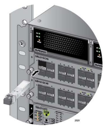
Figure 92. Inserting an SFP or a CSFP Transceiver
